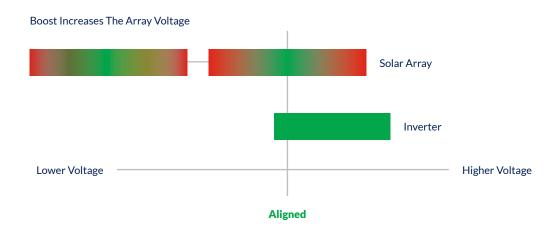
By maintaining the correct voltage range, asset owners can maximize energy transfer from the solar array to the inverter.
