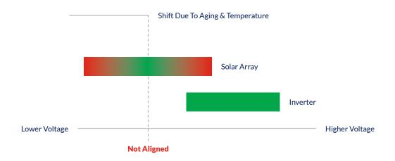
The solar array's peak power voltage and the inverter's MPPT range are no longer aligned, resulting in a loss of energy production.
